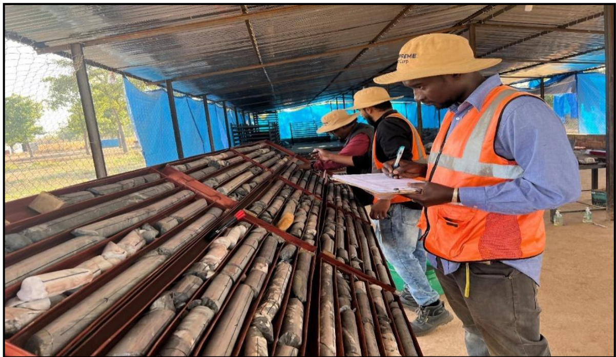
Figure 23. A view of the core logging activities.
