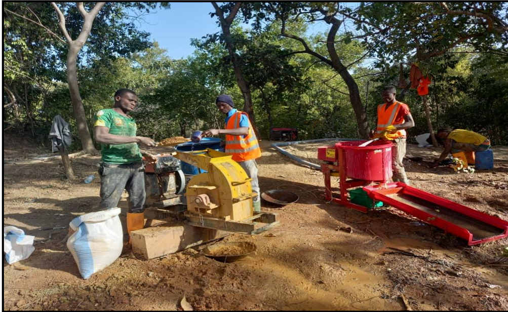
Figure 17. Washing and gravity concentration of the auger samples using the Gold Kacha.
