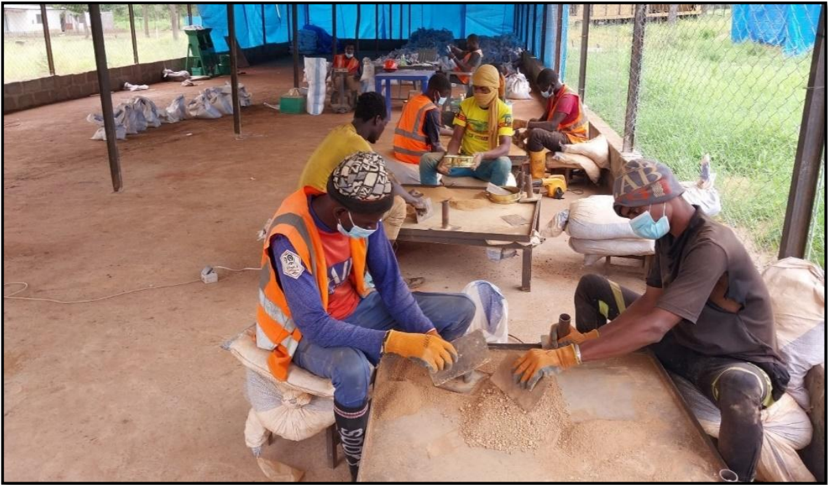
Figure 11. Photograph showing the sample preparation activities in the core shed.
