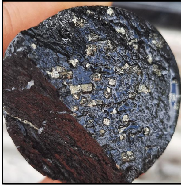
Figure 20. A section view of the core sample showing euhedral pyrite crystals in carbonaceous phyllite.
