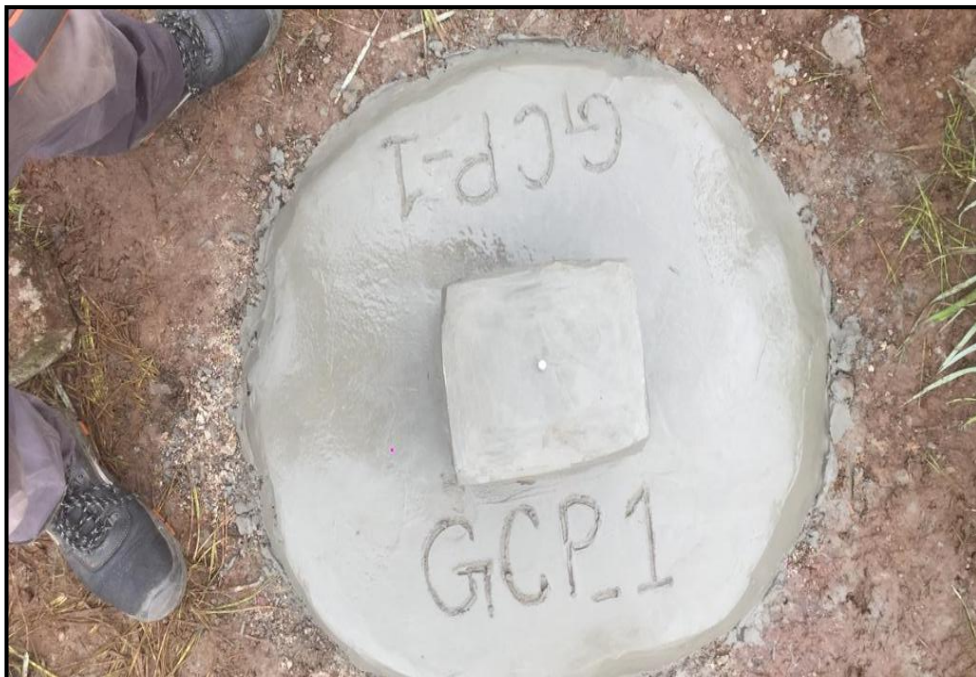
Figure 26. Top view of the Ground Control Point (GCP-01), established inside the camp.
