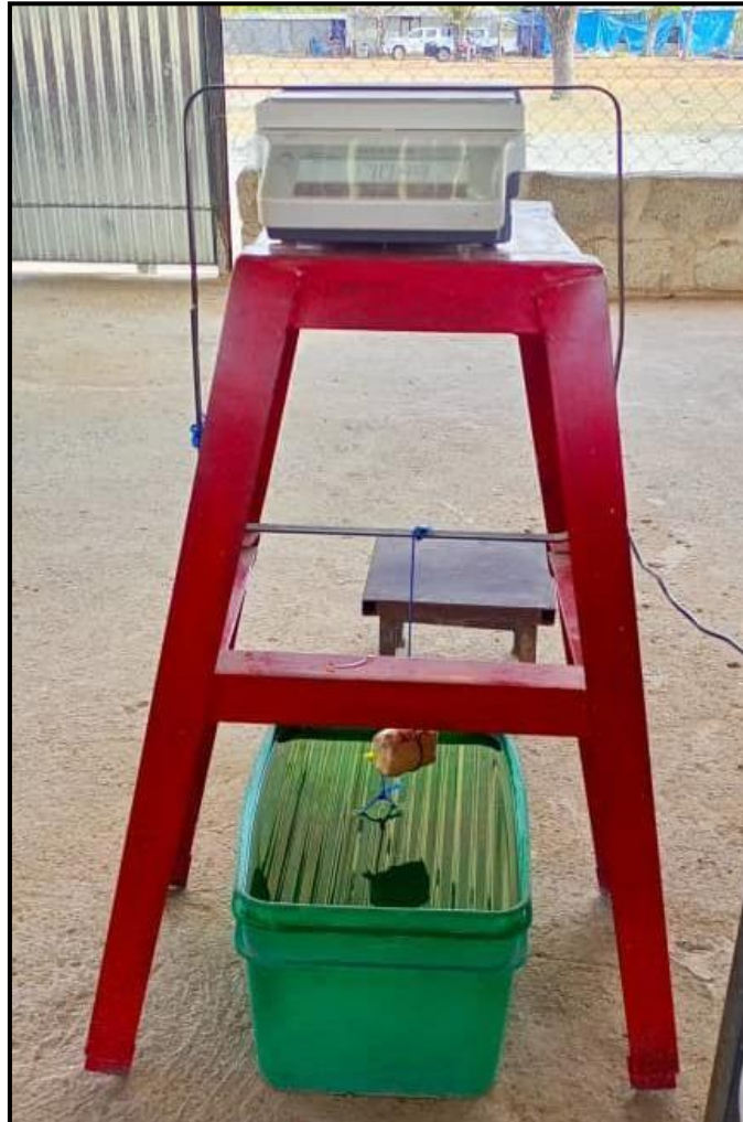
Figure 9. Water displacement apparatus for specific gravity measurements.
